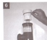
6 Retire o anel O'ring
